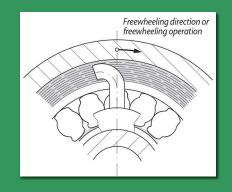
inner rings reduces, the lifting force also reduces. Before achieving synchronous running, the sprags are brought safely to rest on the inner ring and are ready to lock. This guarantees immediate torque transfer once the synchronous speed has been reached. The hydrodynamic sprag lift-off enables a virtually wear-free freewheeling operation.
